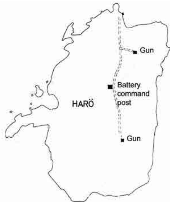
Partial battery plan for the Järnavik (Tärnö) battery showing two of the three guns. This battery was located on two islands, one with two guns and the battery command post. The other island (not shown) had one gun and an emergency battery command post. (Leif Högberg)
